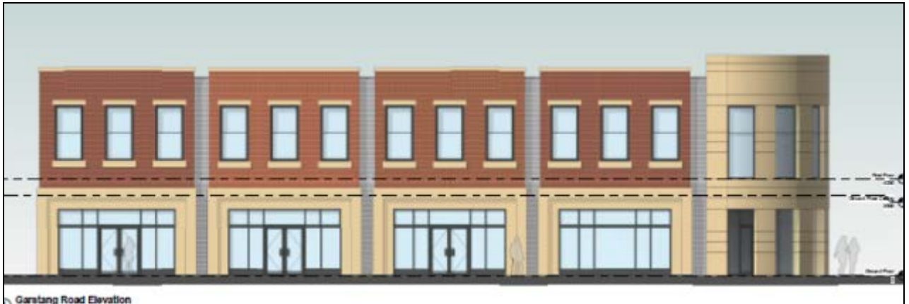
The revised design (Garstang Road elevation), breaking up the elevations into smaller units
